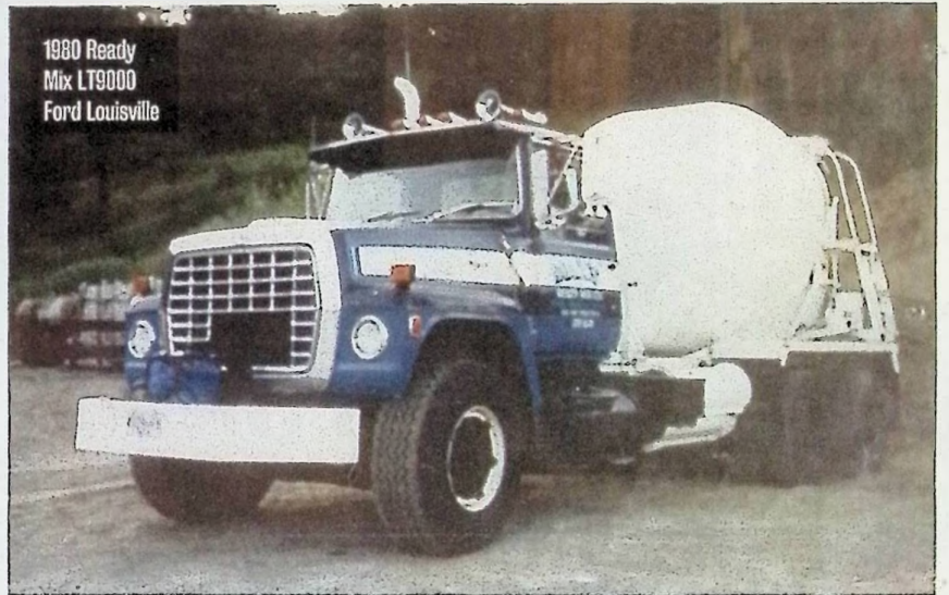
1987 Ford Louisville LT9000 truck came with 18 speed Road Ranger or Spicer transmission, 425 Cat engine, Jake brake, and 44,000 Bogies.
