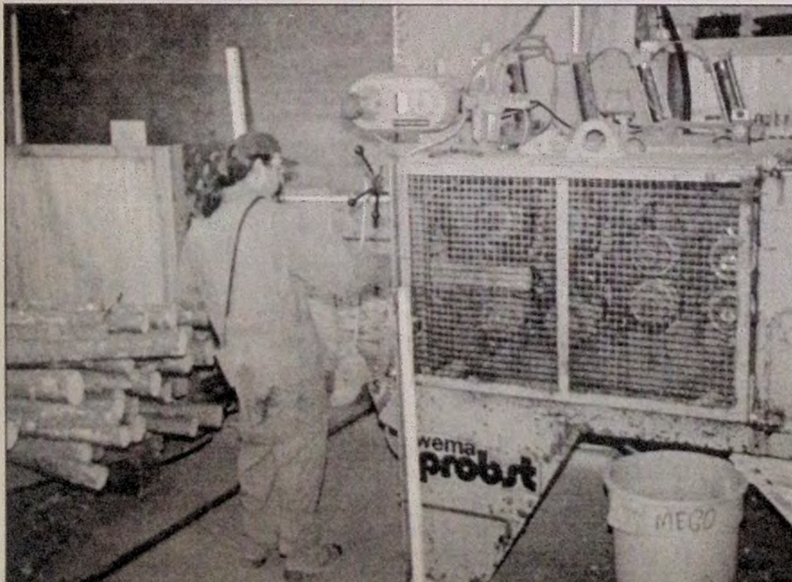
The dowelling machine above accepts posts and both peels and cuts posts to a uniform diameter. Each post is fed into the machine by hand, and it automatically continues through to a sorting deck.
