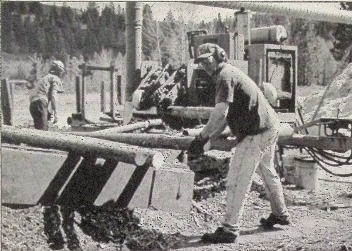
One of the new pieces of equipment at Mego Wood Products is the post peeler shown above. Posts are fed into it from photo right and come out the other side white and cleaned of bark.
