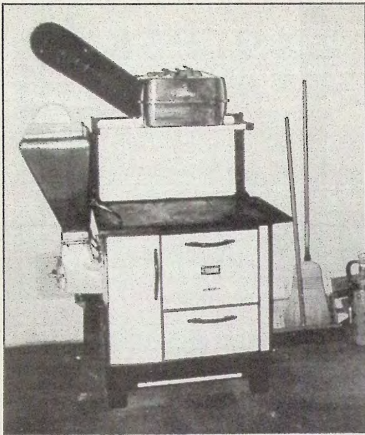
The appliance above is a sawdust burner. Sawdust was poured into the hopper at left and was fed through the bottom of the hopper into the firebox of the stove.
