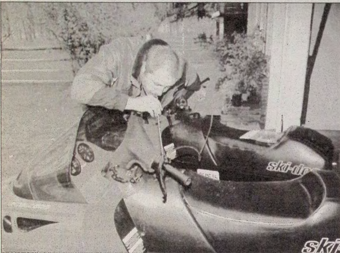
Tom Steele demonstrates the use of his invention, The Blow and Go Siphon. As he blow into the specially designed device, gasoline is transferred from one gas tank to another. Not only is this device convenient, it is healthier as no gasoline enters the mouth of the person doing the siphoning.
