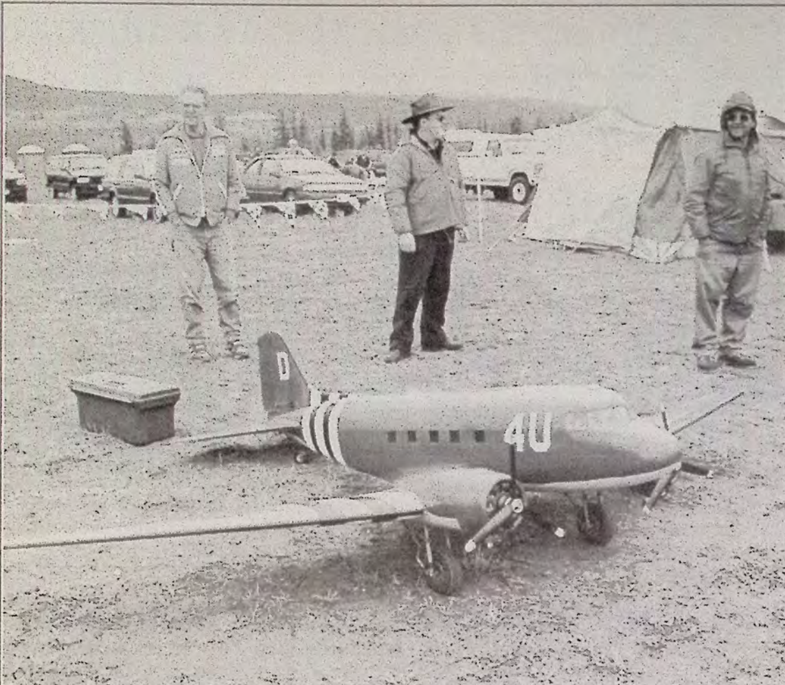
This aircraft is a twin-propeller scale model of the C-47, a transport plane used by the American military in WW 2 and Korea. It was built by owner Chuck Bower (center) of Whidby Island, Washington. It flies on two 2.2 cubic inch gasoline engines and weighs 42 pounds.
