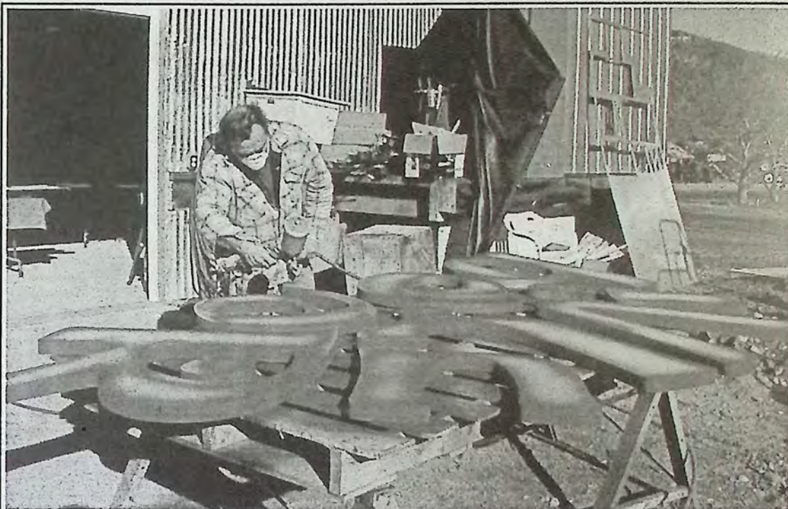
Cornel Hanson sprays paint on laminated foam dimensional lettering for a major sign.
