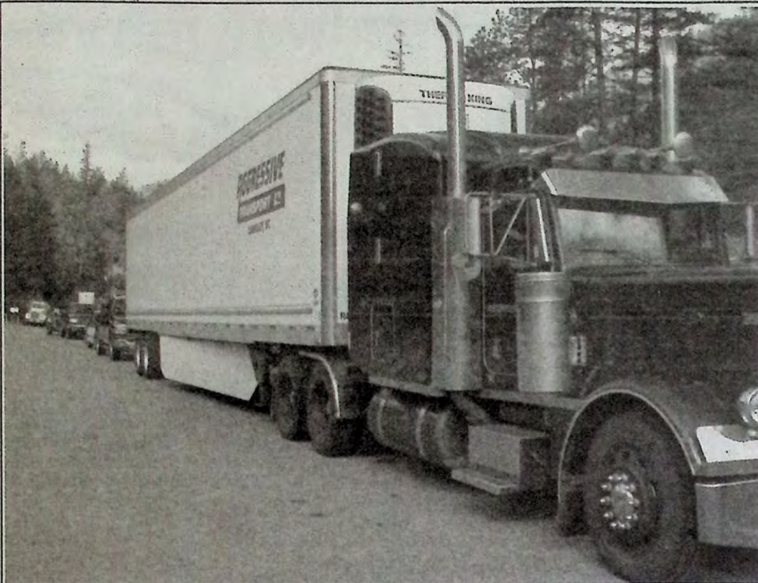
A sign of things to come? This Aggressive Transport Ltd. trailer at the Yellow Lake road block is sporting skirting that reduces wind resistance, thereby increasing fuel economy. Jim Jansen of Aldergrove drives this rig from there and advised that the skirting is law in California. He hadn't bothered to remove the skirting since returning from a recent trip across the border. Interestingly, another Aggressive Transport Ltd. trailer spied at the Yellow Lake road block a few days later did not sport the skirting. Photo: Arlene Arlow
