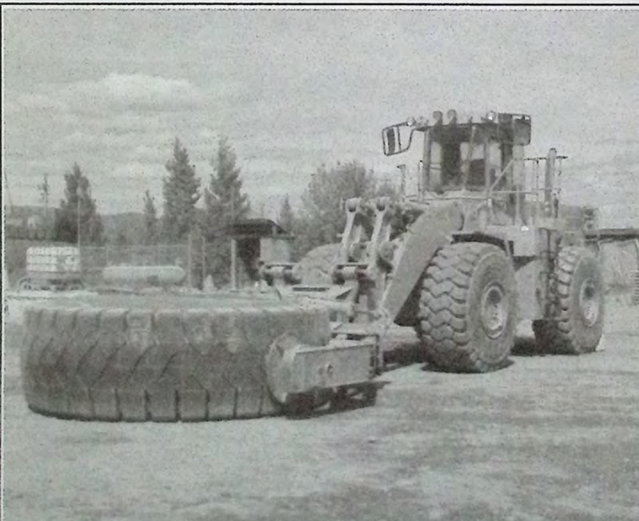
A specialized mine site requires specialized equipment - like this tire mover/changer. *
