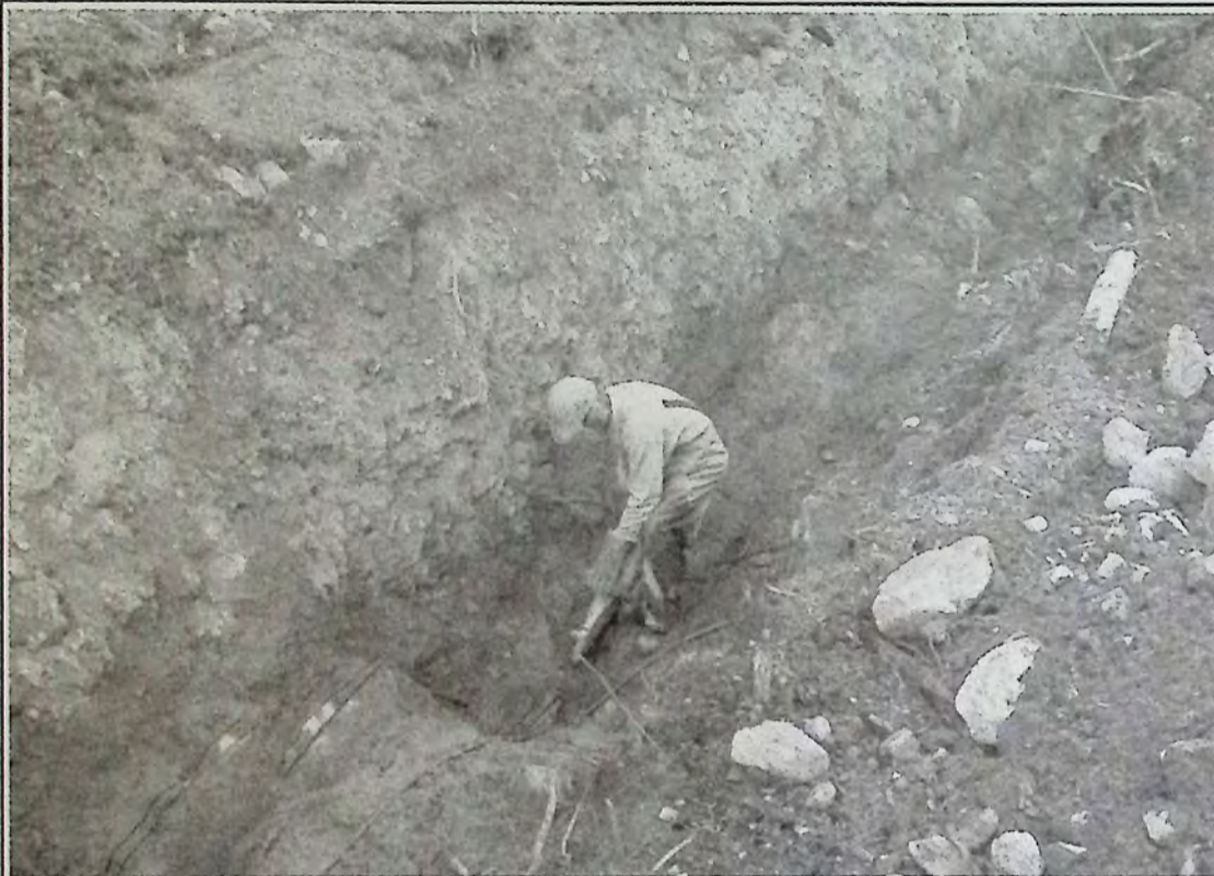
Trench sample cutting at Goldcliff's Panorama Ridge Gold property near Hedley. - photo submitted
