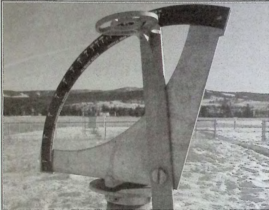
This device, the Alidade, allows one to sight a distant object and use line of sight to perform a task, for example, measure the cloud base at night. Photo: Brenda Engel
