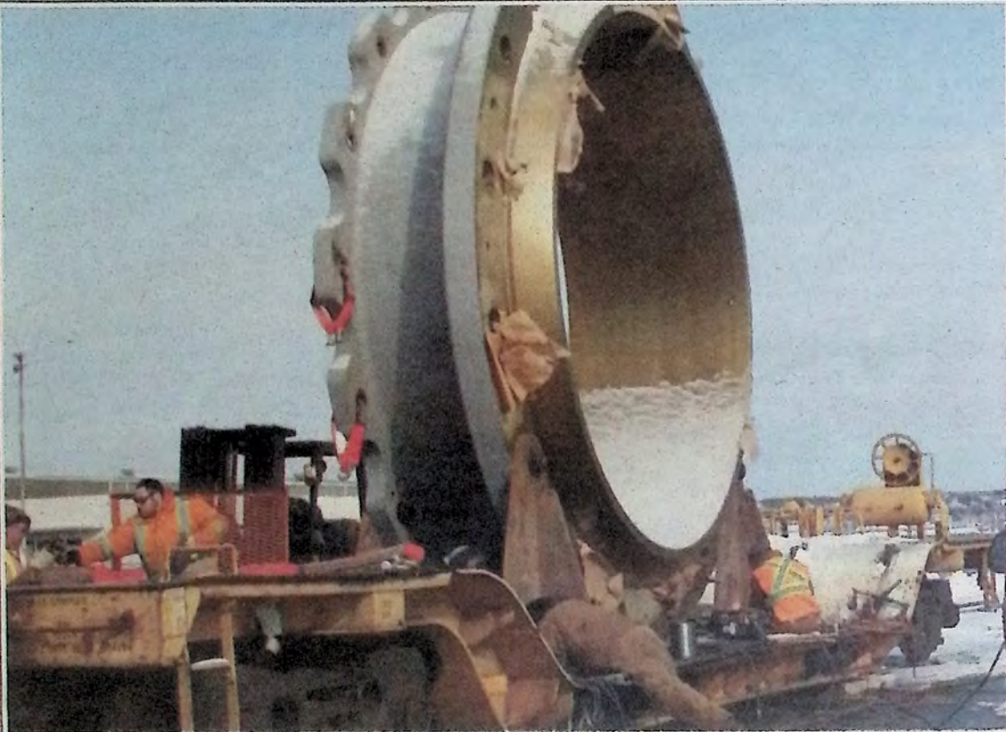
This is part of the new crusher heading for Copper Mountain Mine near Princeton. Once assembled, the High Performance Raptor 2000 will be one of only four such crushers in the world. - photo submitted
