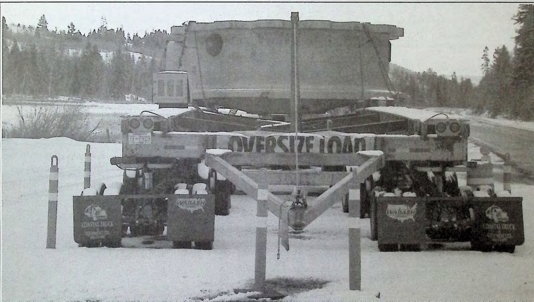
Now that's what we call a w-i-i-d-e load. A part of the new Raptor 2000 secondary crusher for Copper Mountain Mine sat at the pull out at Kidd Lake last week. This view is from the very back of the unit built to haul one piece of the giant machine. The back of this unit is connected to another semi tractor rig used to "push and brake" this one. Photo: Bob Marsh www.marshphotography.ca
