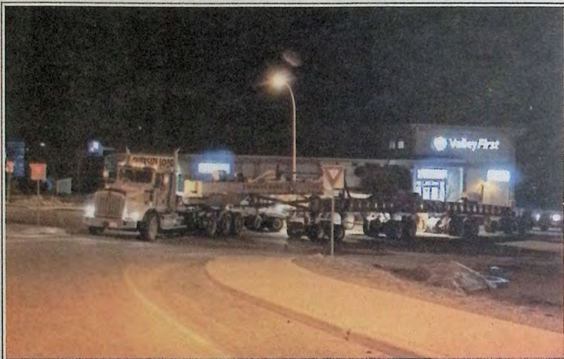
The lower mainframe of the Raptor 2000 secondary crusher makes the corner at Bridge Street and Highway 3 as it was hauled last week on a special transport vehicle to the Copper Mountain Mine for assembly. Photo: Copper Mountain Mine
